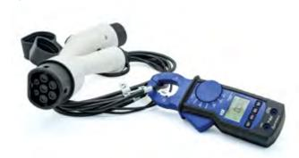
To measure current in L1, L2, L3, N and PE and in CP and PP while the vehicle is charged
